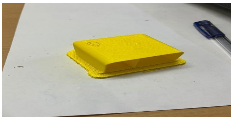
Figure 2 3D printed prototype of the customized chalk piece and duster holder fabricated using PLA material through FDM technology, demonstrating the successful conversion of the CAD design into a functional physical model.
