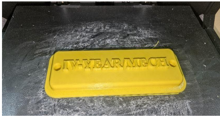
Figure 4 3D printed prototype of the customized Nameplate fabricated using PLA material through FDM technology, demonstrating the successful production of a personalized component from the developed CAD model.
